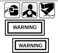
Do not work on hydraulic lines or fittings when system is pressurized. Hydraulic fluid under pressure can cause personnel injury. Depressurize brake system by stepping on the brake pedal several times to bleed off the hydraulic pressure. Make sure brake pressure gauge indicates zero.
